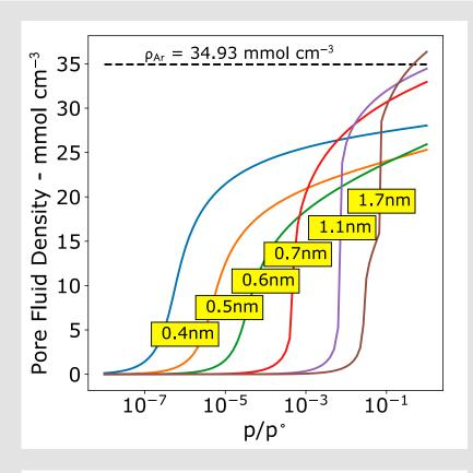
Figure 1: A kernel, a series of theoretical isotherms generated using an NLDFT model (left). Note how fluid density varies with pore size, an effect further illustrated for argon (below). At coarser pore sizes calculated density values converge to that of the bulk fluid.
