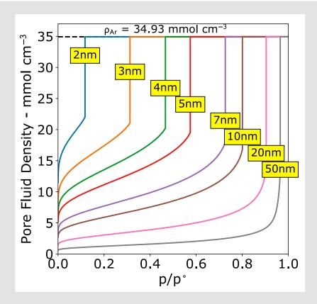
Figure 2: Model isotherms generated using BJH, which assumes that the condensed sorptive exhibits the same density as that of the bulk fluid and as a result is less accurate at finer pore sizes.
