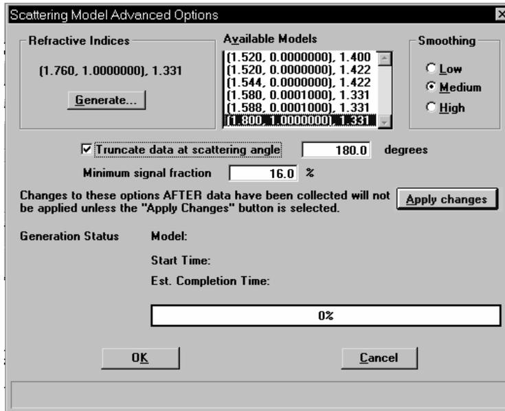
Edit the value in the **Minimum signal fraction** field, then click **Apply changes** to recalculate the particle size distribution with the new minimum signal fraction.
