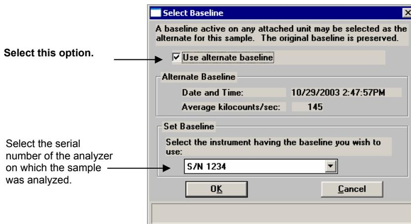
6. From the drop-down list, choose the SediGraph on which the sample was analyzed. If you have multiple SediGraphs installed on the computer, be sure to choose the correct one.
